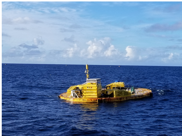
Figure 1. The Wave Powered Adaptable Monitoring Package aboard the Fred. Olsen Bolt. Courtesy of P MEC
