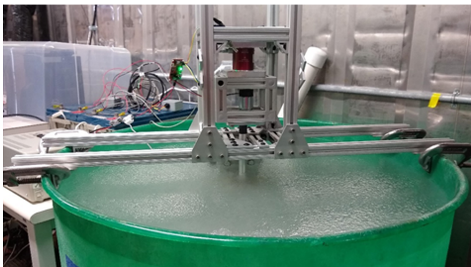
Figure 7. Bearing test stand in Arctic Laboratory with grease ice at surface
