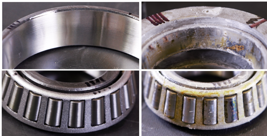
Figure 8. New steel tapered roller bearings (left) and after 1000 hours seawater exposure (right). Orientation is the same for both pictures
