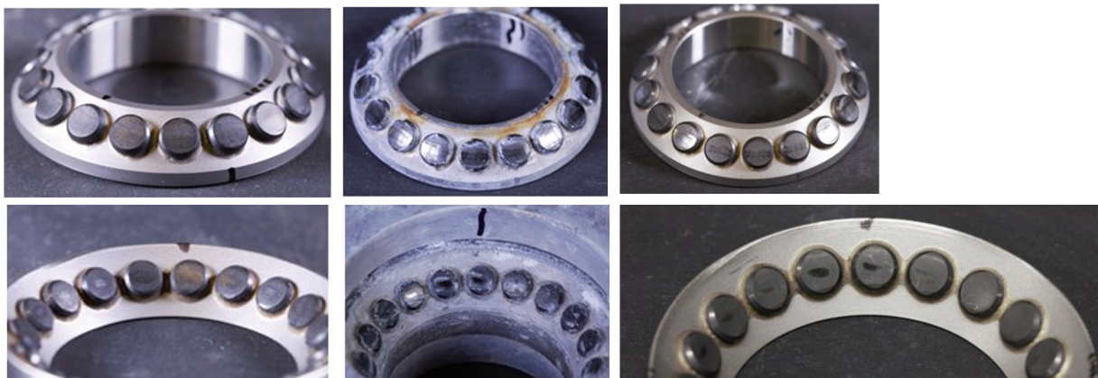
Figure 10. Inner race (top) and outer race (bottom) photographs. New PCD bearings (left), after running for 1,000 hours (middle), and after an acid wash (right). All pictures are taken from the same orientation.
