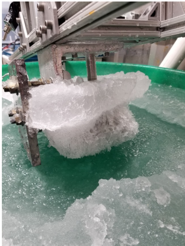
Figure 13. The PCD bearing after 450 hours of running with ice buildup in the bearing
